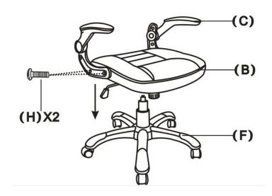
Note: Do not fully tighten bolts in Step 3 to make for easier assembly in Step 4
